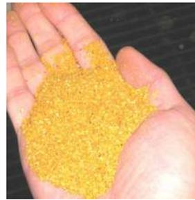
2. Grind samples to pass through a 20 mesh sieve. Mix ground material thoroughly before sub-sampling. Carefully weigh out 20-50g subsample.
